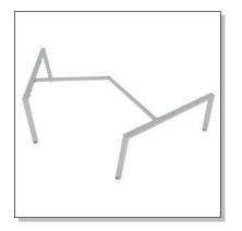
Place 1st outer Rail into correct position on 2 sets of Legs.
