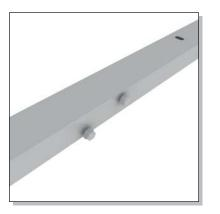
Position **Bolts** loosely on all the **Legs** leaving enough room for the **Rails** to fit.
