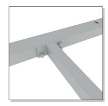
Tighten **Bolts** with the **Rail** in place at the correct height.
